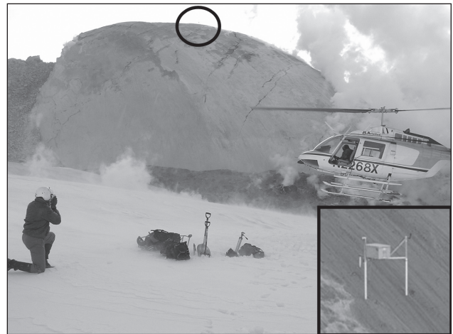
[USGS photo, Jan 14, 2005. Circle is where an instrument package (inset) was dropped to measure the volcanic activity. The package lasted 36 hours until it was destroyed in an explosion.]
